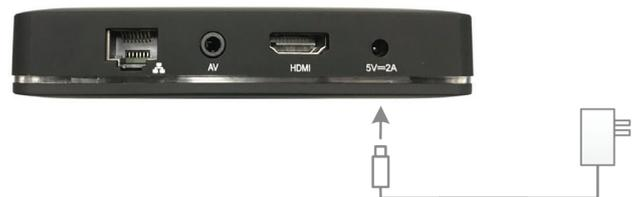
**Warning!** The Amigo 7X must only be used with the supplied power adapter.
